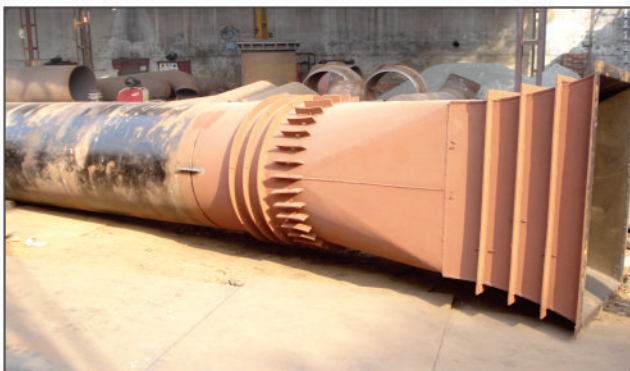
Bell Mouth with connecting Penstock Pipe
