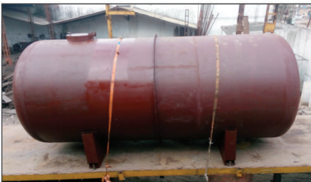
Horizontal Storage Tank as Boiler Auxiliary
